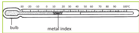
Fig 8.17 (a) A diagram of a minimum thermometer.
