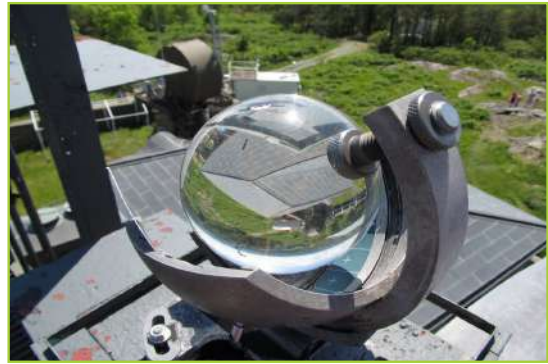
Fig 8.75 A Campbell Stokes sunshine recorder.
